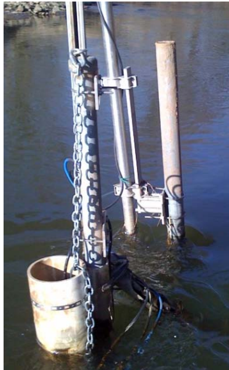
Figure 2.3. Photo of the assembled sensor station at Oxford and similar to Camp Cardinal Road. The Nitratax sensor is located on the farthest pipe.
